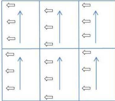
7. Roll material is stretched slightly during the manufacturing process. At the job site, the installer should unroll all cuts and allow to relax overnight. A bare minimum of two hours is required. Shaking the material once it is unrolled can help it to relax.
