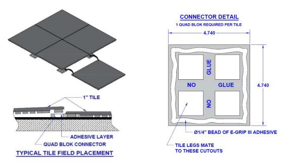
Note: Adhesive spills must be removed while still wet. Use a dry rag to pick up the majority of the adhesive. Wipe the remaining residue with a rag dampened with mineral spirits, followed by a rag damp with water to remove the mineral spirits. Cured adhesive can only be removed from surfaces by mechanical means, such as scraping or sanding.
